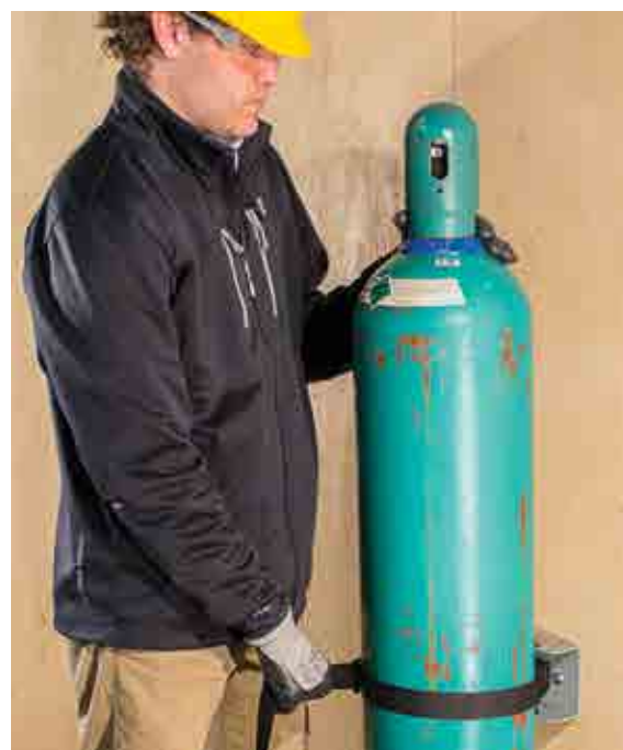
Secure gas-cylinders to wall or bench to prevent tipping.
